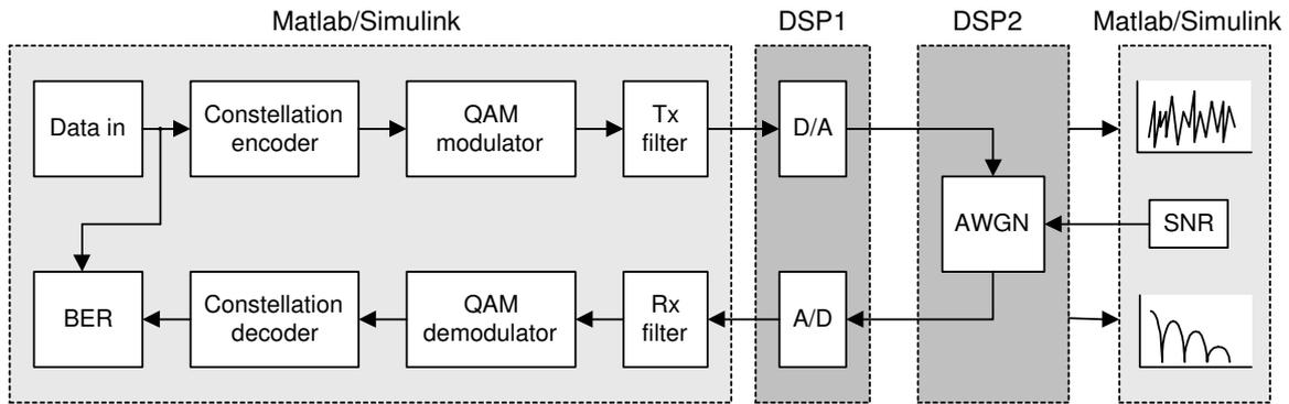
**Figure 5. The functions of the QAM Modulator-Demodulator experimental set-up.**
