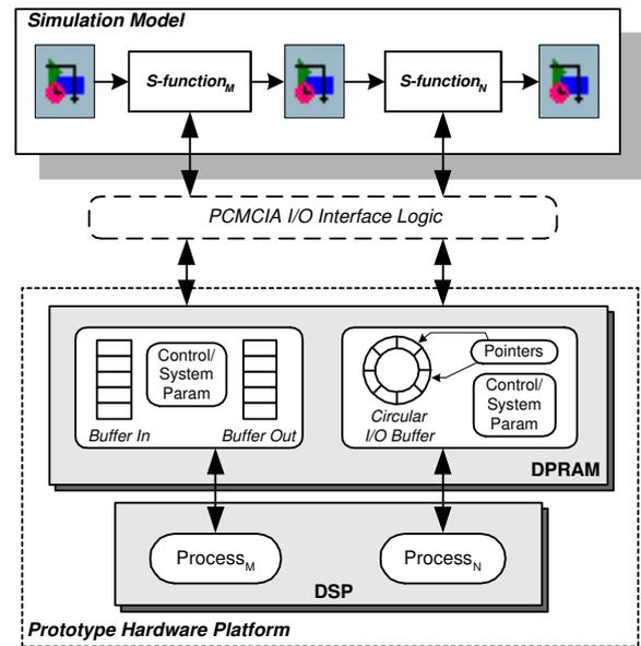
**Figure 4. Runtime communication between Simulink and DSP modules.**
