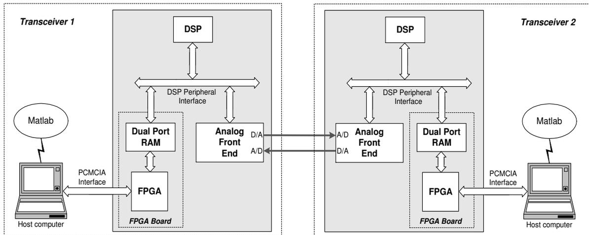
Figure 2. The architecture of the prototype environment.
