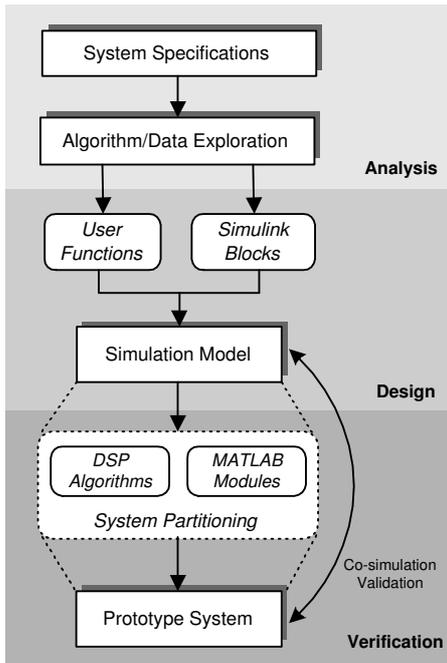
**Figure 1. The prototype design methodology.**
