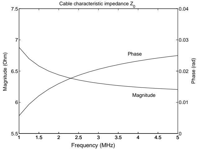
Figure 4: The  $Z_0$  in the frequency range of 1 to 5 MHz
