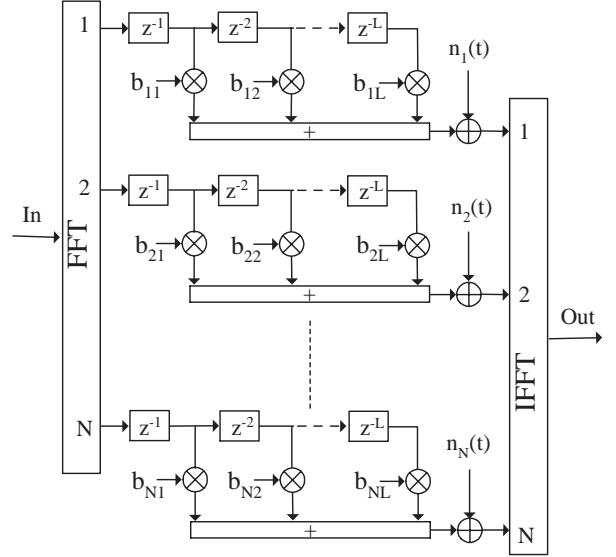
Figure 1: Multipath channel model using multiple FIR filters. Each FIR filter represents a single subchannel.
