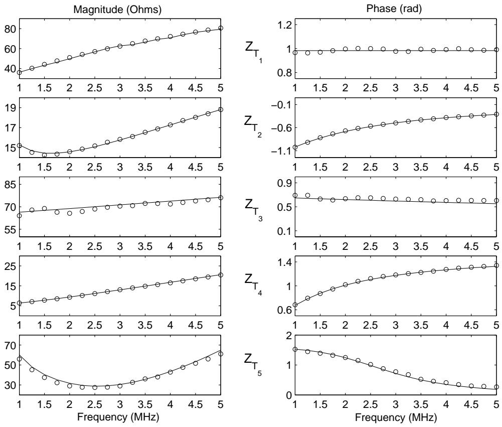
Figure 5: Theoretical and estimated termination impedances in the frequency range of 1 to 5 MHz
