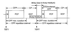
**Fig. 1** *CFP/CP time-sharing mechanism* B = Beacon
