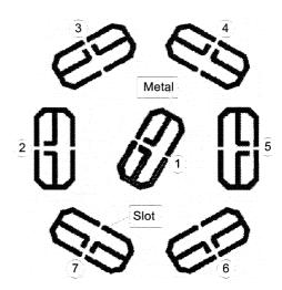
Fig. 1: The seven-elements antenna array.
