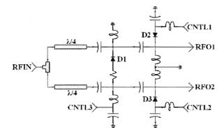
Fig. 2: The feeding network circuit.
