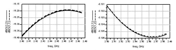
Fig. 5: S-parameters of the single output case
