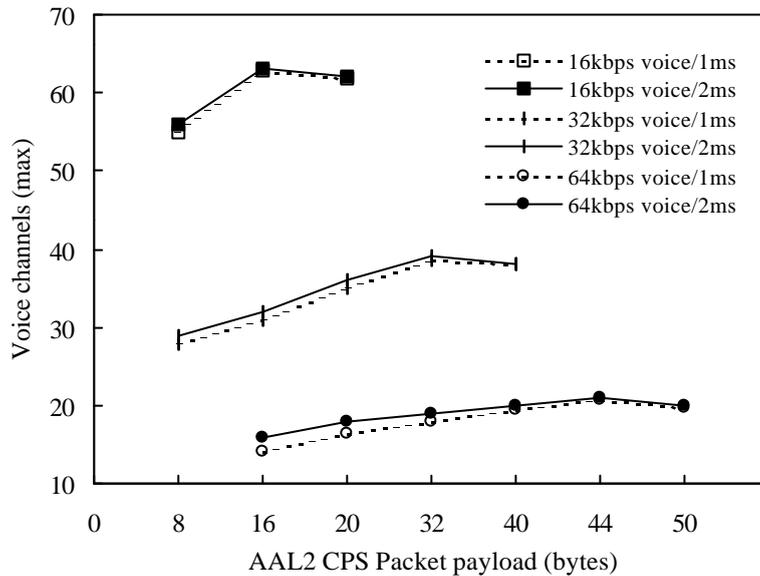
**Figure 4.** Number of voice channels for different size of AAL2 CPS packet payload
