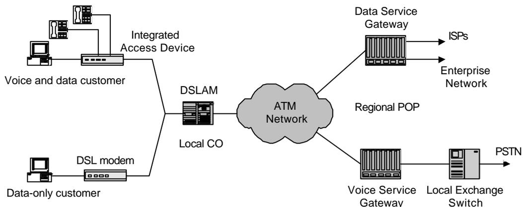
**Figure 1:** Generic architecture for packet voice and data over DSL
