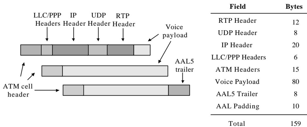
**Figure 2.** Packet format for VoIP/AAL5 connection with 80-byte voice payload
