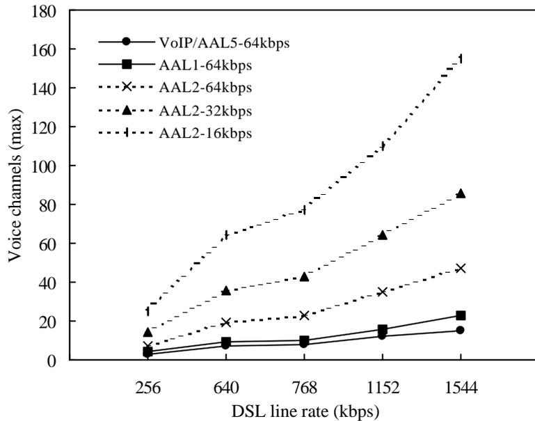
**Figure 6.** Number of voice channels with silence suppression for AAL2
