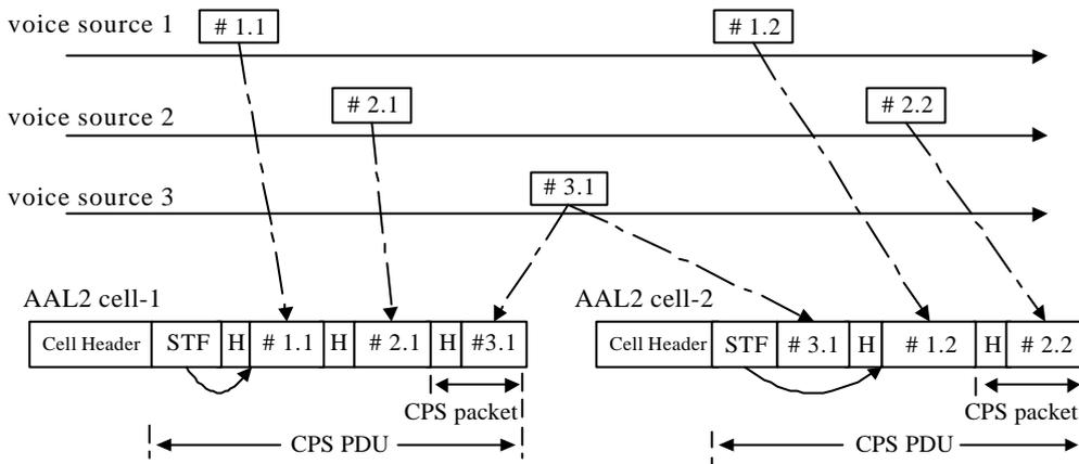
Figure 3: AAL2 cell packing
