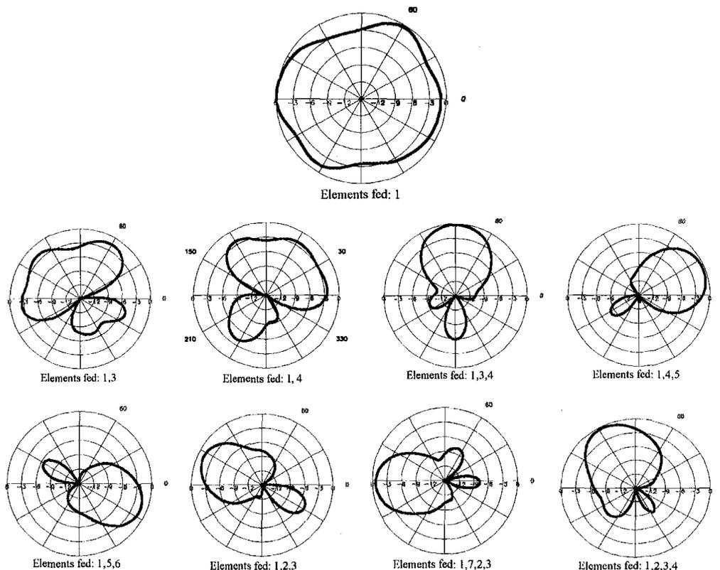
Fig 10: Some of the antenna array azimuth radiation patterns
