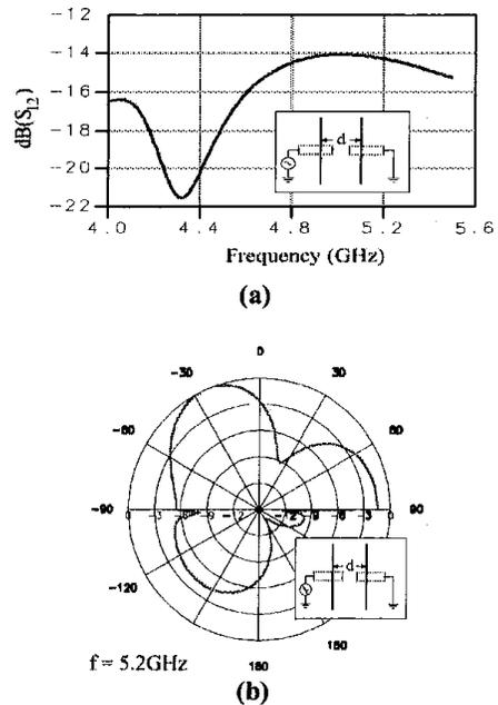
Fig 5: Transmission coefficient parameter  $S_{12}$  (a) and elevation radiation pattern at 5.2GHz (b) between microstrip fed slots ( $d = 20\text{mm}$ )
