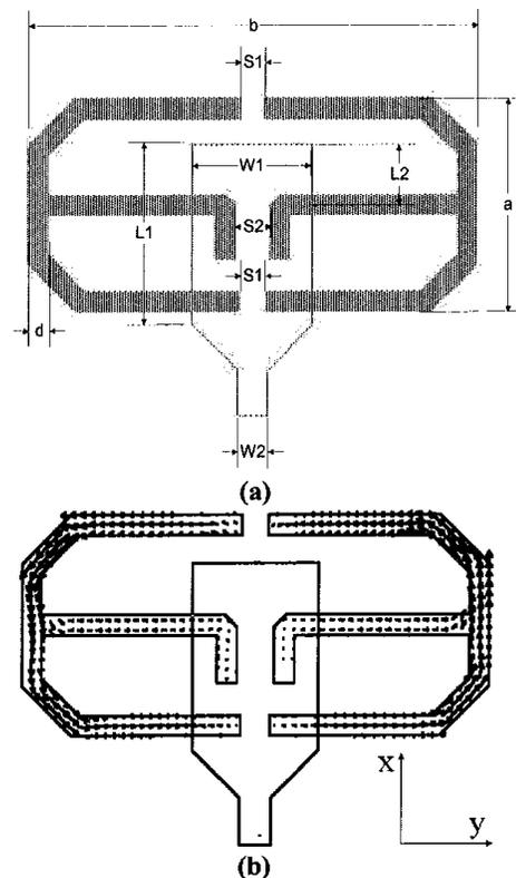
Fig 1: Slot element geometry (a) and current distribution (b) for slot dimensions:  $a=12.52\text{mm}$ ,  $b=18.6\text{mm}$ ,  $d=0.8\text{mm}$ ,  $W1=5.6\text{mm}$ ,  $W2=2.5\text{mm}$ ,  $L1=7.7\text{mm}$ ,  $L2=3\text{mm}$ ,  $S1=1.1\text{mm}$ ,  $S2=1.42$  at 5.2GHz
