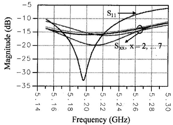
Fig. 9: S parameters of the proposed array
