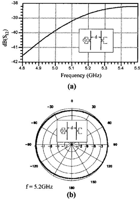
Fig 3: Impedance coupling (a) and azimuth radiation pattern (b) of closely spaced non-resonant dipoles ( $d=20\text{mm}$ )
