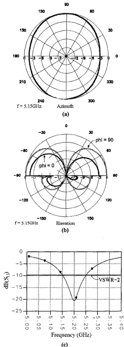
Fig 2: Slot element azimuth (a) and elevation (b) radiation patterns, and return loss (c) for the slot of Figure 1.
