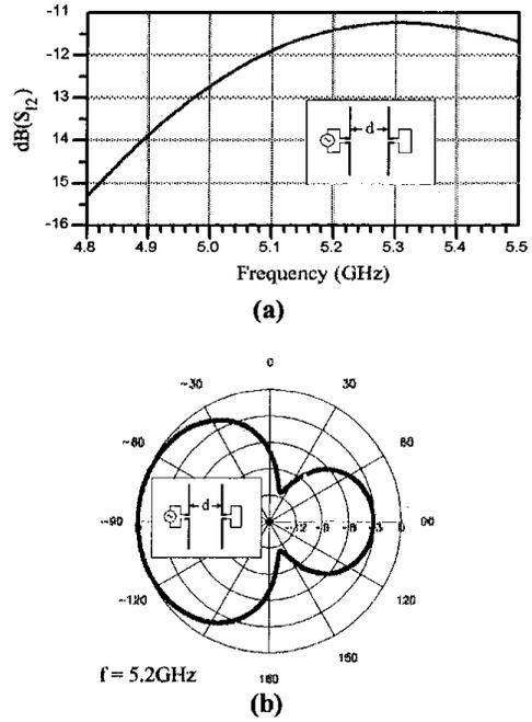
Fig 4: Impedance coupling (a) and azimuth radiation pattern (b) of closely spaced resonant dipoles ( $d=20\text{mm}$ )
