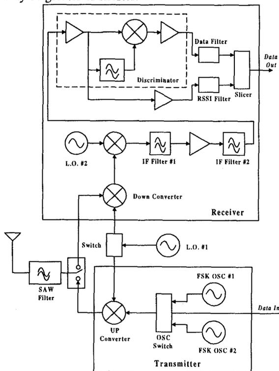
Fig. 2. The RF module block diagram
