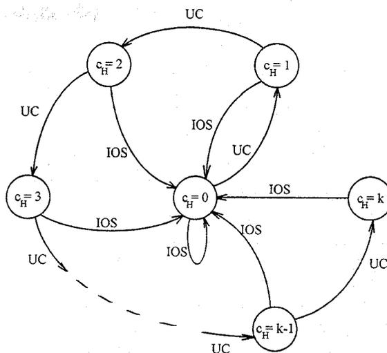
Fig. 2. The VIRUS Tx state diagram
