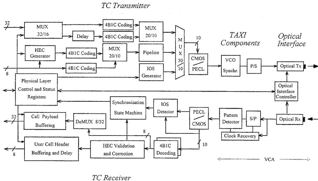
Fig. 5. The VIRUS interface block diagram.
