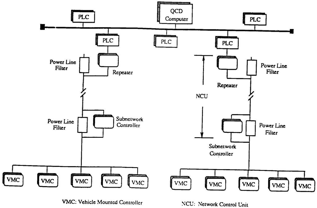
Fig. 2. The Distributed Network Configuration
