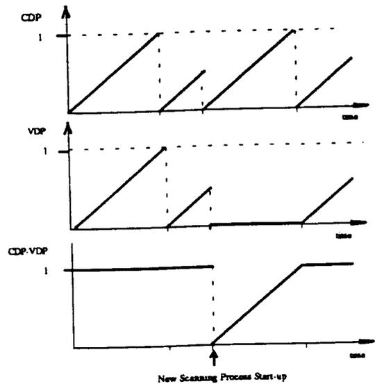
Fig. 7. The Memory Pointers versus time during a new scanning process start-up.
