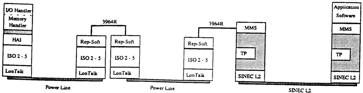
Fig. 3. The Network Protocol Stack.
