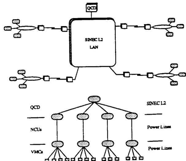
Fig. 1. The Distributed Network Model.
