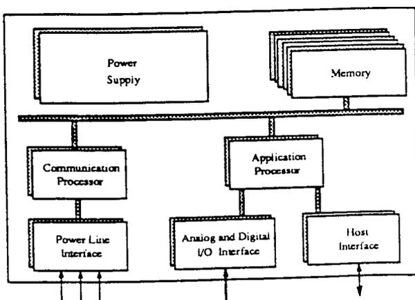
Fig. 4. The PLNode Hardware Architecture
