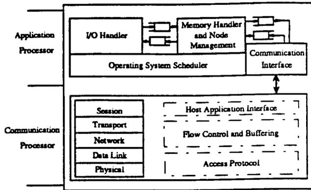
Fig. 5. The PLNode Software/Protocol Architecture
