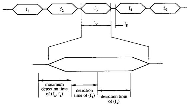
Figure 6. The '5-tone' selective signalling system.
