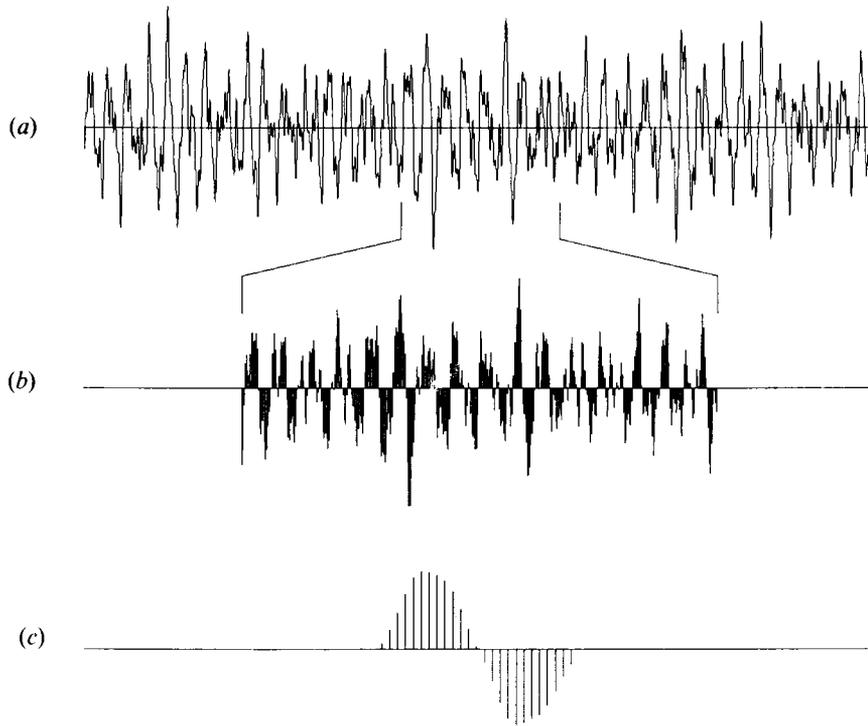
Figure 2. Example of the proposed method: (a) the received signal; (b) the sampling process; (c) the averaging results.
