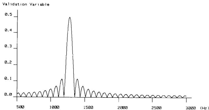
Figure 5. Validation variable versus frequency (expected frequency: 1275 Hz).
