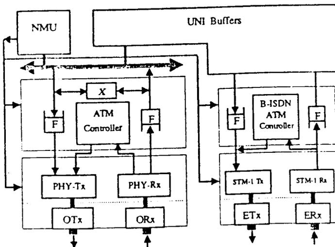
Fig. 3. The UNI - CPNode Architecture.
