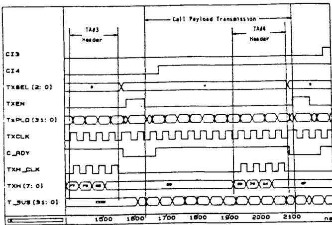
Fig. 5. Cell assembly timing diagram.
