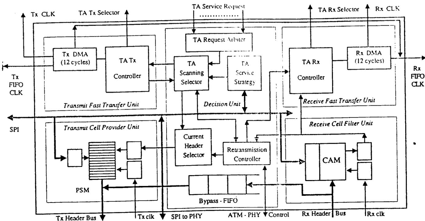
Fig. 4. The Medium Access Controller Block Diagram.
