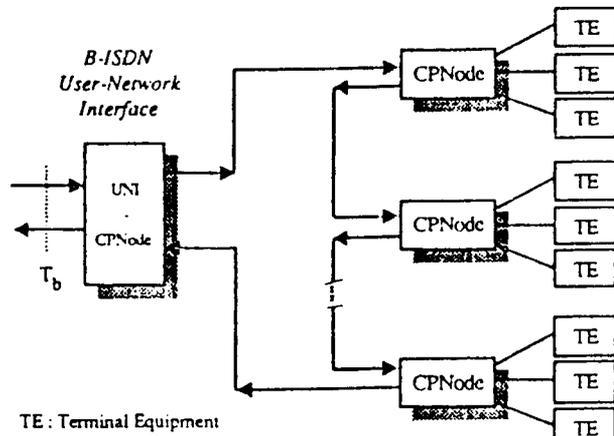
Fig. 1. The Customer Premises Network Architecture.
