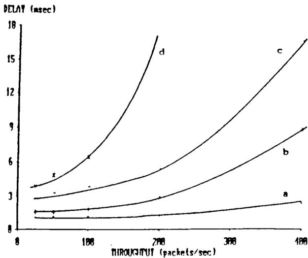
Fig. 3. The Read channel Throughput-Delay characteristics.
