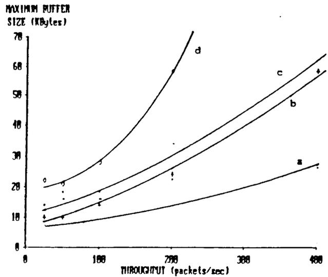
Fig. 5. The Read FIFO buffer maximum length.
