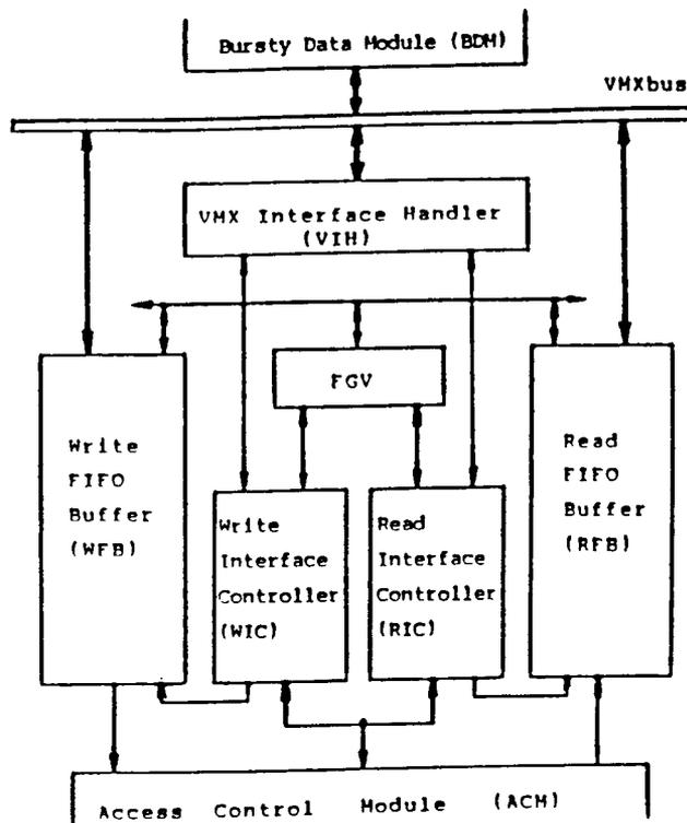
Fig.1. The functional diagram of the I/O Packet Buffer.
