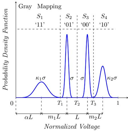
Fig. 1. Voltage distributions of a 4-levels cell.
