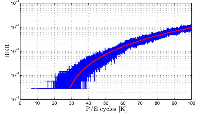
Fig. 3. MLC NAND Flash experimental BER versus P/E cycles.
