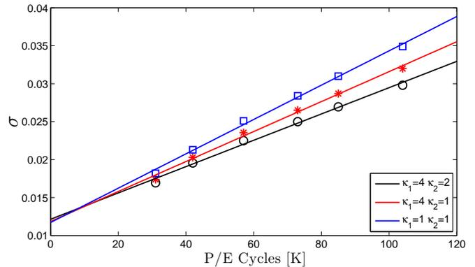
Fig. 7. The relation of introduced noise and the P/E cycles.
