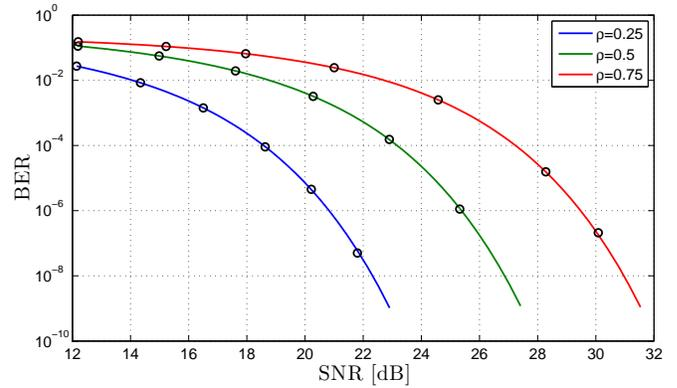
Fig. 6. BER as a function of SNR for non-equally probable symbols.
