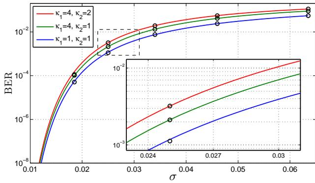
Fig. 4. BER as a function of  $\sigma$  for non-equally probable symbols ( $\rho = 0.25$ ).
