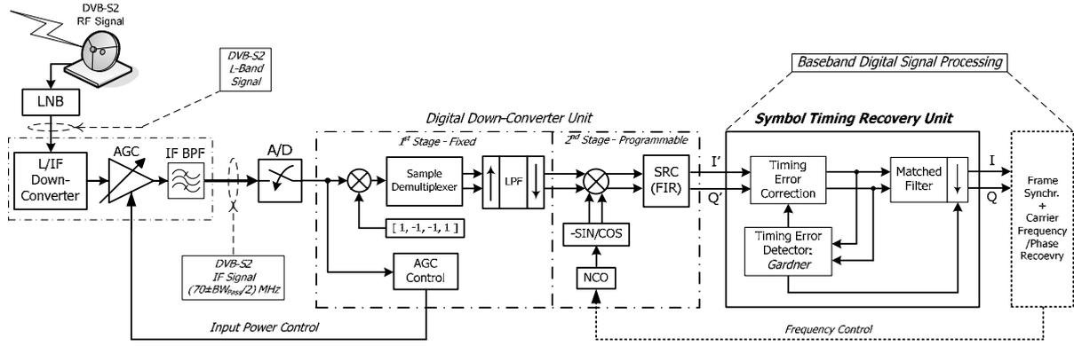
Figure 1: A DVB-S2 Receiver Architecture
