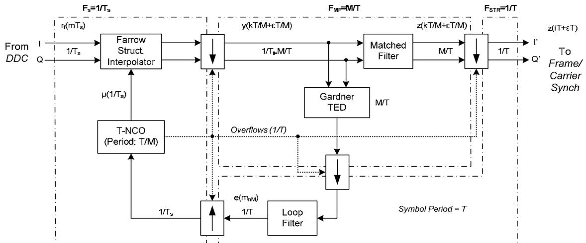
Figure 2: Closed-Loop STR using the NDA Gardner TED
