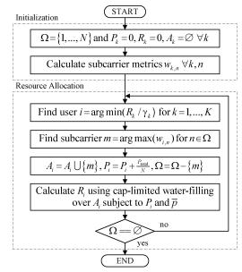
Fig. 1. Multiuser resource allocation algorithm.
