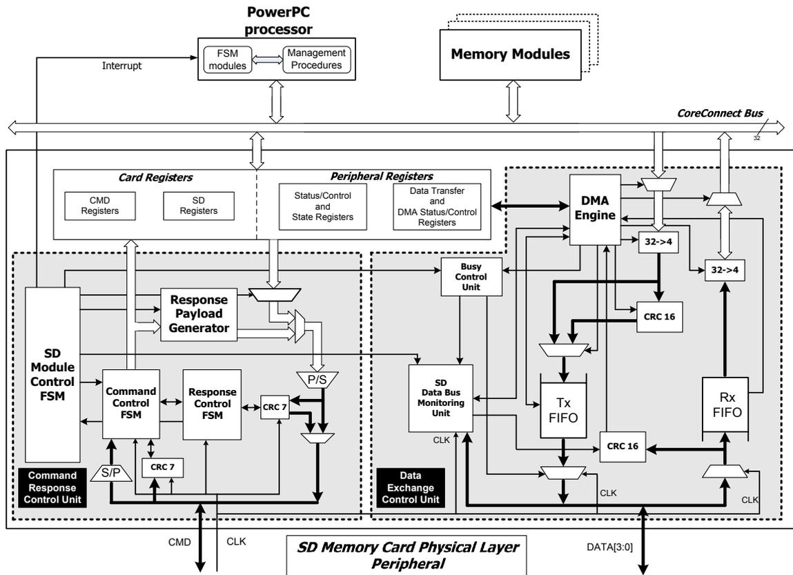
Figure 2. SD Memory Card Interface Peripheral Architecture.
