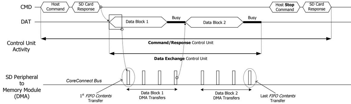
**Figure 3. An example of the ‘Write Multiple Block’ Command in the SD Memory Card Prototype.**
