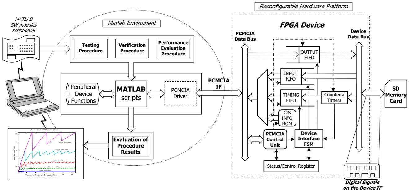
Figure 4. SD Card Interface Testing Environment.
