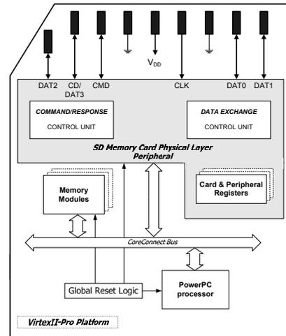
Figure 1. SD Interface Prototype Platform Architecture.
