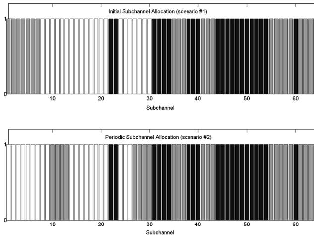
Fig. 3. Subchannel allocation of the three virtual links. Each shading represents a different virtual link.
