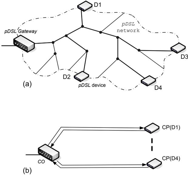
Fig. 1. A *pDSL* network and the equivalent DSL topology.
