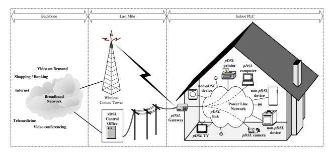
Figure 1: pDSL Service Structure.
