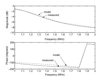
Figure 7: Measured and modelled response of the experimental network (1-2 MHz).
