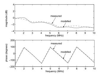
Figure 5: Measured and modelled response of a 53.3m cable line.
