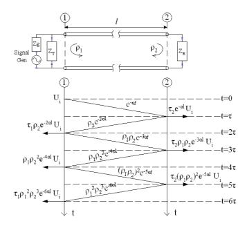
Figure 1: Timing diagram of signal propagation on a cable line.
