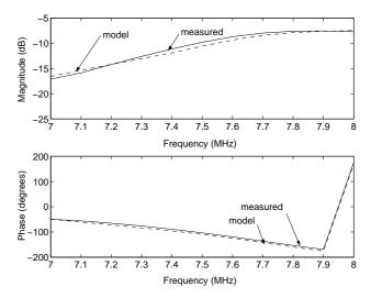
Figure 8: Measured and modelled response of the experimental network (7-8 MHz).
