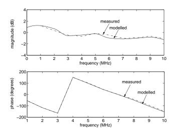
Figure 4: Measured and modelled response of a 22.3m cable line.
